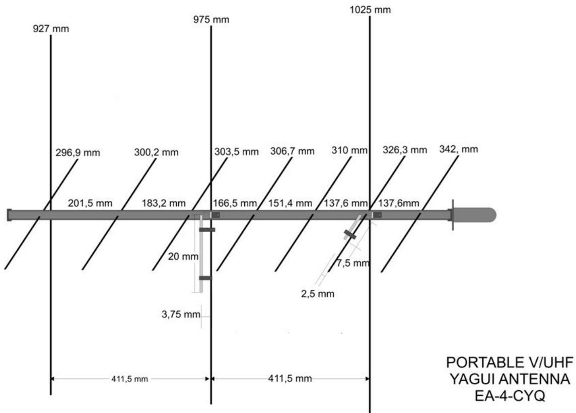
Figure nº1: Scheme of a dual-band portable antenna
