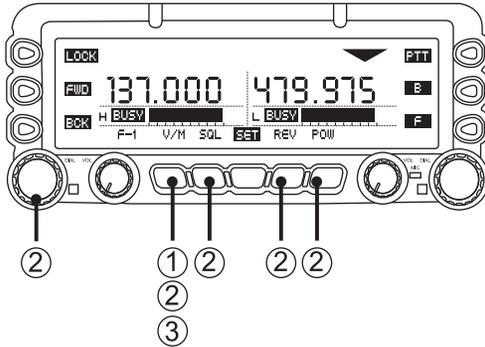
① Press and hold the **[V/M]** key for two seconds to display the “Memory Edit” window.
