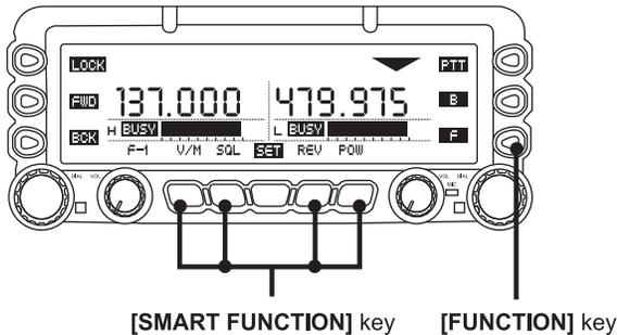
Pressing the **[F]** key repeatedly will change the function command of each **[SMART FUNCTION]** key as shown in the following tables. It is easy to recall and perform a desired operation. The current function of each key is shown in the display above the button.
