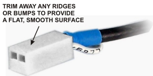
Figure 8. Preparing TMP Cable for Installation.
