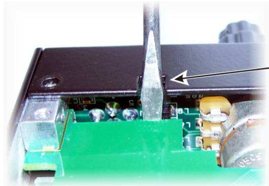
Figure 7. Separating the Front Panel Assembly from the Chassis.
