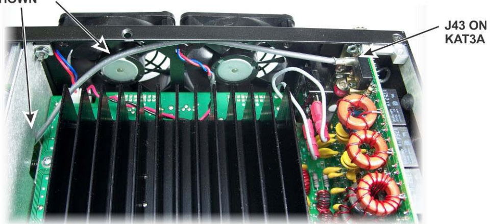
Figure 29. Optional KRX3A Antenna TMP Cable to KAT3A.
