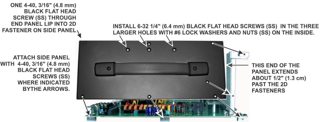
Figure 66. Mounting Left Side Panel.
