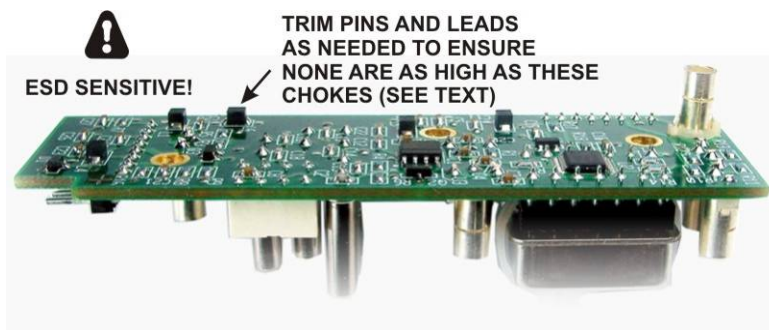
Figure 79. Checking Lead Lengths on KREF3 Board.
