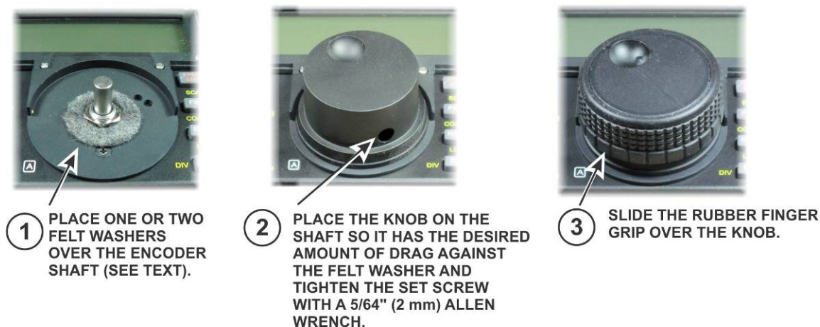
Figure 20. Mounting the VFO A Tuning Knob.
