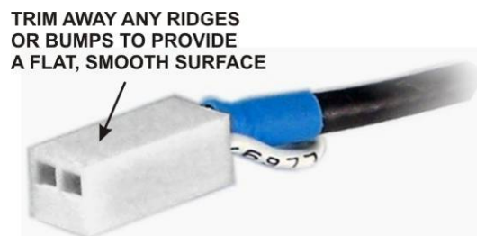
Figure 54. Preparing the KXV3B TMP Cable for Installation.
