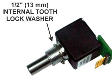
Figure 12. VFO A Encoder Assembly Preparation for Installation.
