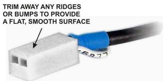
Figure 8. Preparing TMP Cable for Installation.
