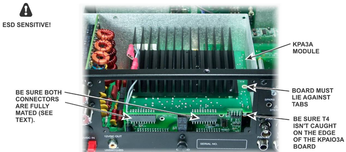
Figure 15. Mounting the KPA3A Module.
