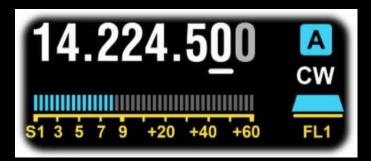
Adjacent to each VFO's numeric display is its ID (A in blue, B in green) and operating mode. Mode icons or the [MODE] switch can be tapped to change modes. See <u>OPERATING MODES</u> for per-mode operating instructions.
