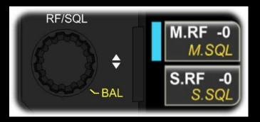
The default value for the RF gain controls is 0 (no reduction in RF gain). Counter-clockwise rotation of the knob increases attenuation (reduces gain) from 0 to -60 dB.
