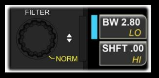
Rotate {FILTER} to adjust receiver filter bandwidth and shift, or hi-cut and lo-cut.
