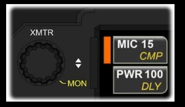
• During CW use, many operators will leave <WPM> (internal keyer code speed) as the selected function of {XMTR}. You can tap the knob or its LCD labels to select the other functions as needed: <PTCH> (sidetone pitch), <PWR> (power output), or <DLY> (VOX delay).
