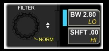
Tap the knob to alternate between <BW> (or <HI> cut) and <SHFT> (or <LO> cut). Hold the knob to select the [NORM] (normalized) passband for each mode. When the passband is normalized, two "wings" appear on each side of the filter graphic as shown below:
