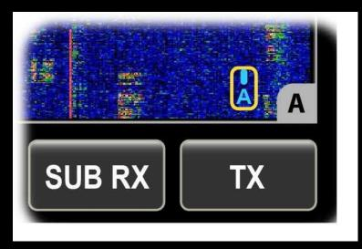
This icon includes a letter to show the current target for mouse-wheel tuning: A=VFO A, B=VFO B, R=RIT/XIT offset. The icon is also color-coded: blue for VFO A, green for VFO B, and white for RIT/XIT.
