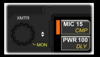
Rotate {XMTR} to adjust often-used transmit functions.
