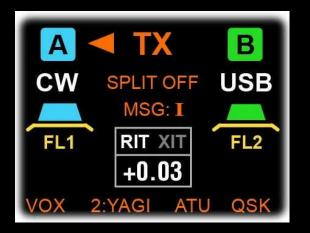
"TX" and its arrows show which VFO is selected for transmit (see <u>USING SPLIT</u>). The VOX icon shows that VOX is on for the current mode (see <u>VOX</u> switch); ATU shows whether the ATU is in-line (<u>ATU</u> switch); QSK shows whether QSK (fastest break-in CW) is in effect (<u>QSK</u> switch).
