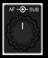
The inner concentric knob, {AF}, sets main receiver AF gain. The outer concentric knob, {SUB}, normally sets sub receiver AF gain. It can also be configured to control left/right channel audio balance (see <u>RF Gain, Squelch, and Main/Sub Balance</u>).
