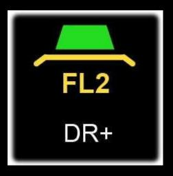
Technical note: The ON setting turns on the ADC's dithering and digital interface randomization, both of which help linearize the ADC in the presence of strong signals. Thus the DR+ icon represents both *Dynamic Range* and *Dither/Random*.
