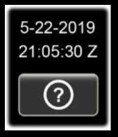
The status area, just above the Info button (<?>) at the lower-left corner of the screen, normally shows UTC date and time. Tapping this text brings up the STATUS DISPLAY button group, allowing
