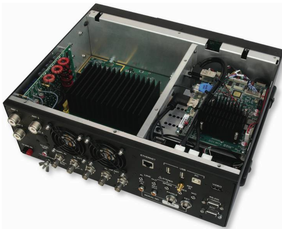
K4 top view with cover removed showing the PA, ATU and single board computer.
