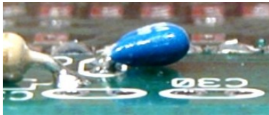
Figure 6. Positioning C39 Against the PCB.
