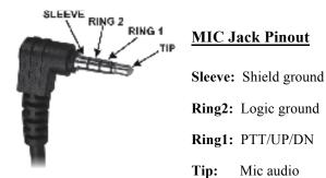
The KX2 will work with many other mics, including "mini" mics intended to plug directly into a computer. Refer to the *MIC BIAS* and *MIC BTN* menu entries to set up the KX2 for use with your mic or headset.
