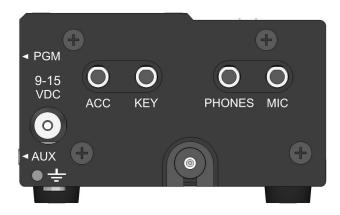
An external power supply or battery can be connected to the 9-15 V jack on the left side panel (see above). The center pin is (+). The plug can be a Switchcraft model S760 or similar (2.1 mm aperture, 5.5 mm dia.). The white striped wire on the supplied cable is (+). Trim the cable to the desired length.
