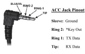
\* For external ampflier keying, the ACC jack's *key out* signal (on *Ring 2*) may also be needed, as described at right. In this case a 4-circuit (TRRS) plug is required.
