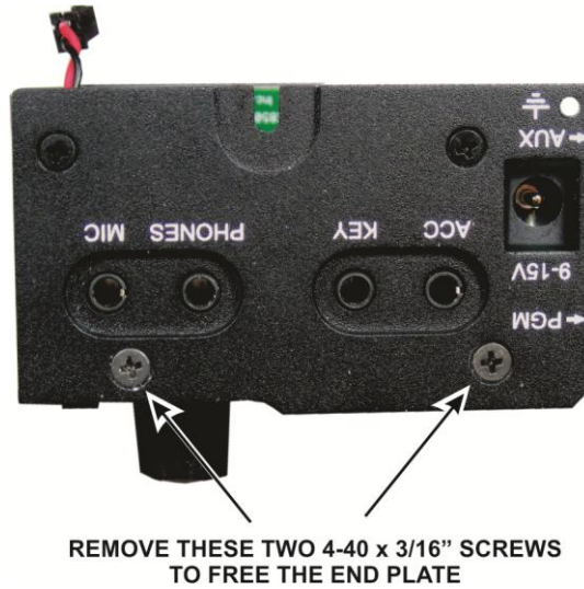
Figure 3. Removing the KX2 End Plate.
