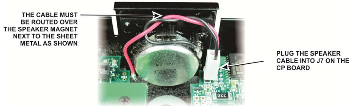
Figure 10. Reconnecting the Speaker.
