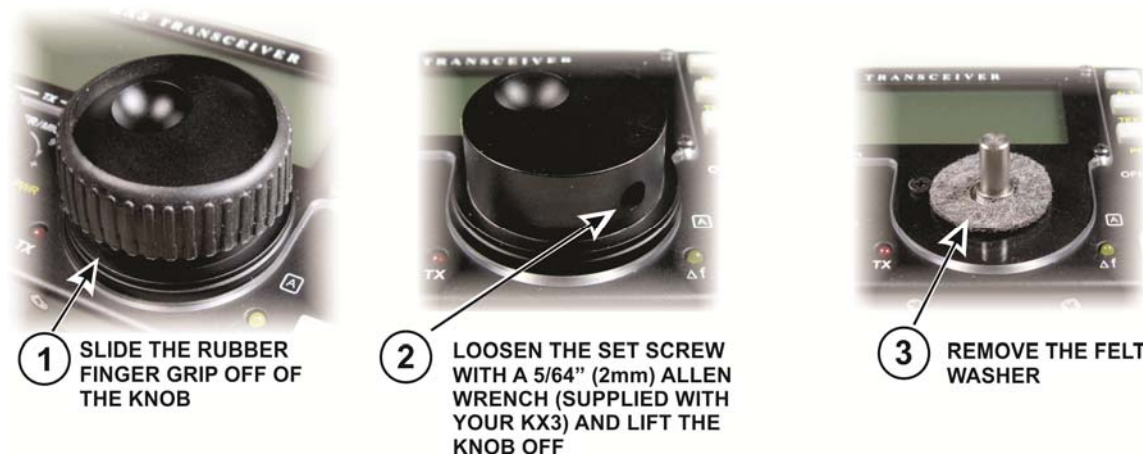
Figure 2. Removing the VFO Knob.
