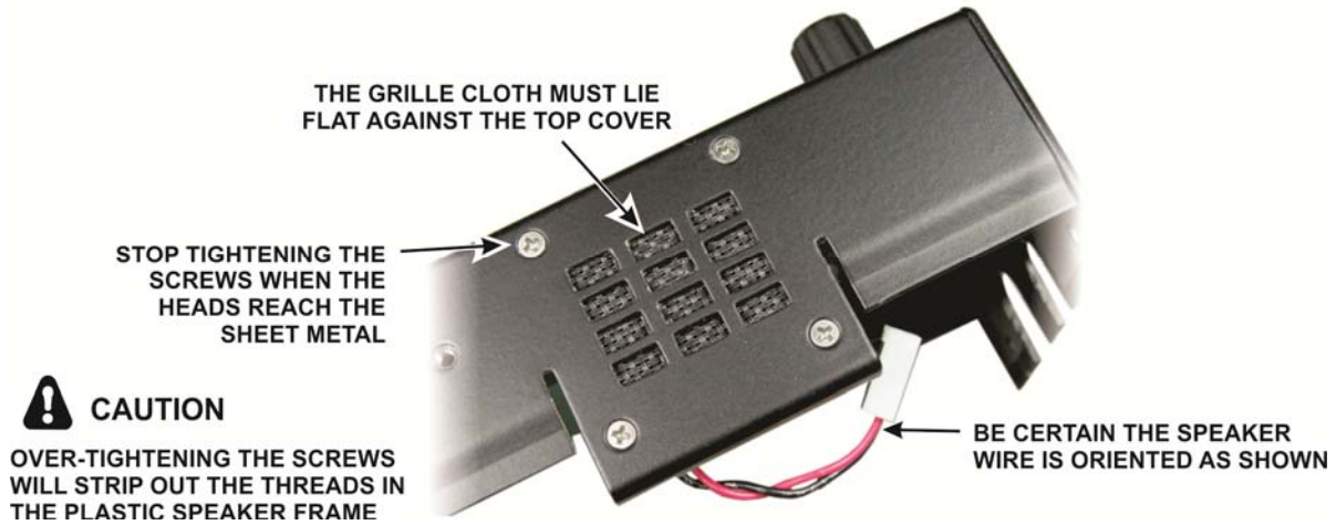
Figure 9. Replacing the Speaker in the KX3.
