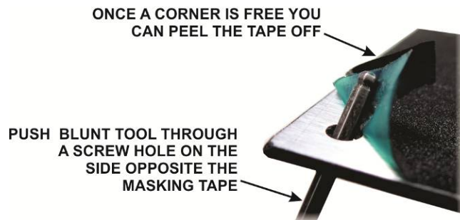
Figure 3. Removing Masking Tape from the Rear Panel.
