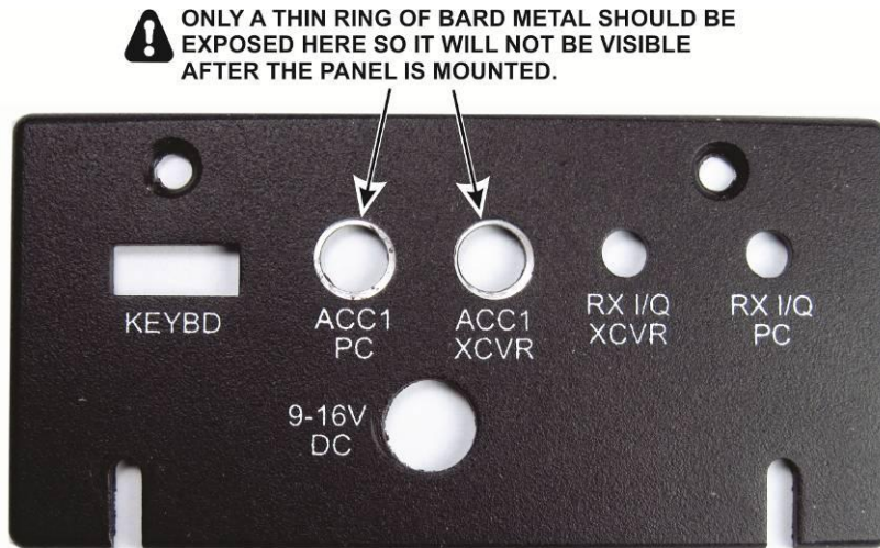
Figure 38. Checking the Grounding Surface on the ACC1 PC and XVCR Connector Openings.
