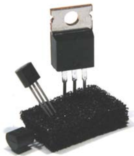
Figure 2. A common antistatic packaging is conductive foam which keeps all of the terminals of a device at the same potential.
