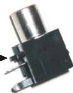
Figure 27. Preparing the RCA Jacks for Installation.
