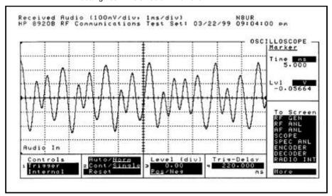
This picture is guaranteed to give a TNC fits. Recall that the demodulator chip used in the most popular TNCs particularly hates this condition -- it wants the high tone to be stronger than the low one. Even if the signal is very strong, the TNC will have trouble decoding it. If the signal is weak, and there's additional noise riding along with the tones, the chances of successfully decoding a packet become very slim.
