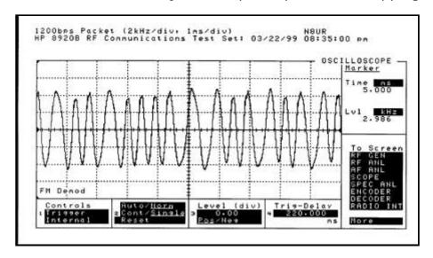
The clipper has chopped both the high and low tones at the same level; there's no trace of preemphasis left. In fact, the low tone is actually a little bit louder than the high tone -- that's probably caused by the other distortion that "hard" clipping introduces.
