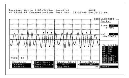
In a perfect world, the two received tones would also be at the same amplitude. Here, you can see that the high tone is somewhat louder than the low one; the transmitter I used for this test boosts the high frequencies a bit more than it should. Within reason, that's not a problem; a twist in the opposite direction, though, is a different matter. By the way, you can click here for details of the test setup I used for these pictures.
