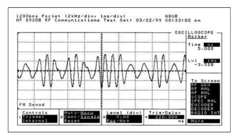
The high tone has nearly twice the amplitude of the low tone; that makes sense since the preemphasis boost is 6dB/octave -- 2200Hz is nearly double 1200Hz. (There's a little bit of distortion visible in the low tones in this picture; I'm not sure where that is coming from -- it may be an artifact of the measurement setup.)
