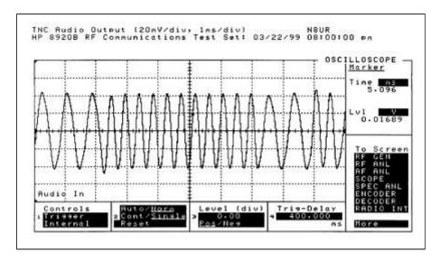
The receiver at the other end of the link recovers these tones, and sends them via its speaker jack to the TNC, where a demodulator (the "dem" part of a modem) converts the tones back to binary form for further processing. For best performance, the tones fed into the demodulator should be at equal amplitudes, or biased a bit toward the high tone. If there's a lot of imbalance (or "twist") in the tone levels, demodulation performance is likely to suffer.
