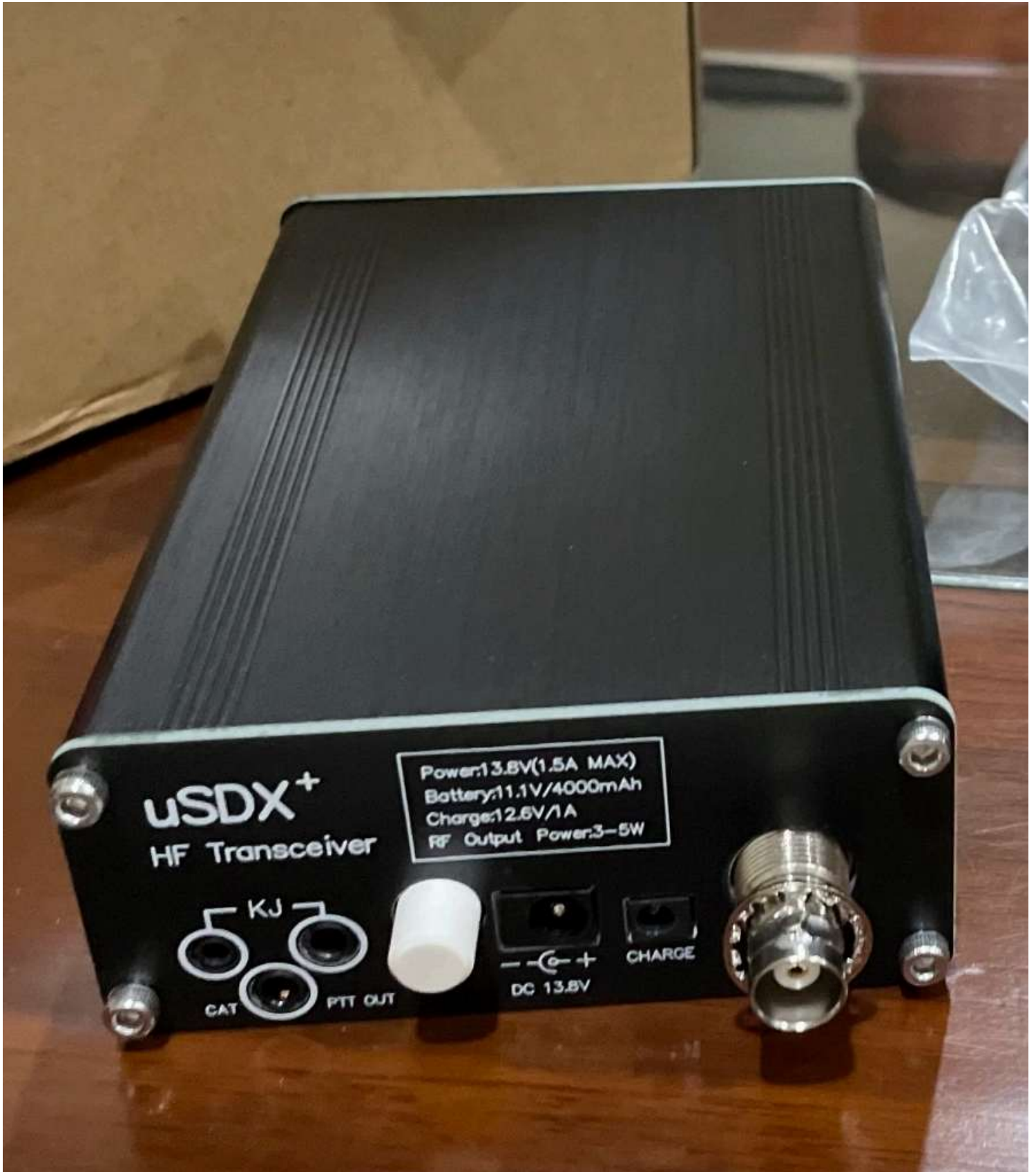
CAT (also PTT signal out) jack underneath the speaker-mic jack (denoted with KJ)
