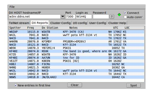
*flcluster* connects to and displays data from DX cluster servers. The three most common server types are AR-← Cluster, CC-Cluster, and DX Spider. The program is designed to work stand alone or as a helper application to fldigi. It can transfer call, mode, and frequency data from a spotted QSO to the appropriate fldigi controls. It can query fldigi for the same items when generating a spot report.
