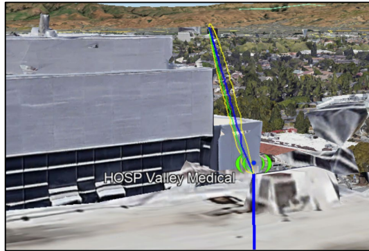
Example: Line of sight radio path between Valley Medical and San Jose hub
