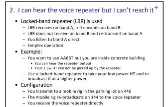
Locked-Band Repeater Example Repeater - AA6BT 146.715 RCV Freq RCV Freq 146.115 XMT Freq 446.500 446,500 RCV Freq RCV Frea 146.115 446.500 XMT Freq XMT Freq 146.715 146.115 XMT Freq Sql Type Tone Tone SQL Sql Type Tone SQL Sql Type Tone Freq 100 100 Tone Freq Tone Freq 100 100 Tone Freq N/A Man SQL Man SQL Sql for no sig
