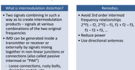
dissimilar metals, etc. May be a combination of fundamental and harmonic frequencies
