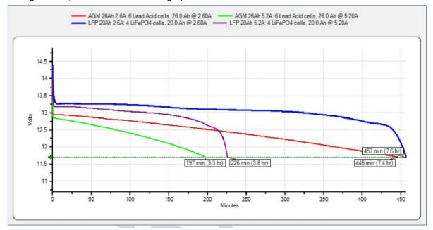
• These results can be summarized and compared to the expected values for the 26Ah AGM battery as interpolated from the datasheet.
