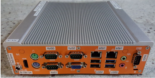
No moving parts (fanless) Mirrored SSD storage Commercial temp range (120F)
